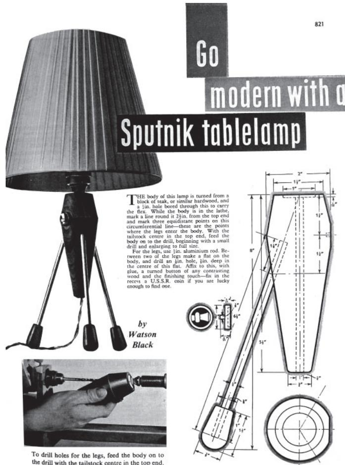
Fig 1. During the 1960s it became increasingly common for do-it-yourself magazines to include measured drawings of home-build projects. Plans for the construction of a table lamp, reproduced from *Practical Householder* August 1961, p. 821
